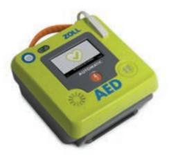
The AED 3 *Automatic* delivers the shock automatically after a three-second countdown. No need to push the Shock button.
